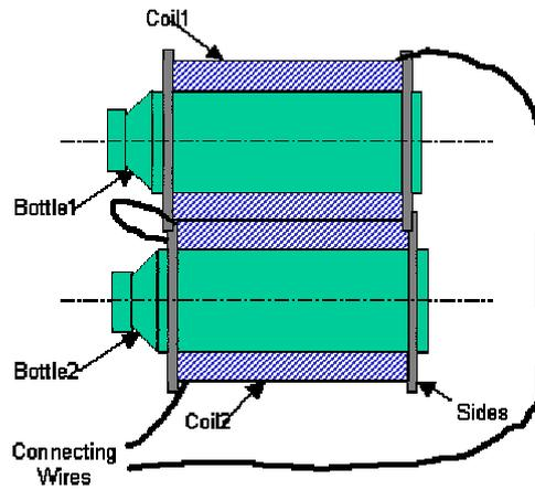
2. Two separate coils are **wound on the same axis around the same bottle**. There must be a wide gap between the two coils because the two polarization fields cancel each other there. They are **connected in series and in opposition** (wound in the opposite direction) to get the same effect
